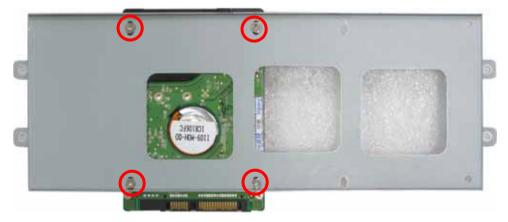
6. Screw on as indication of the picture below Turn the screws.
