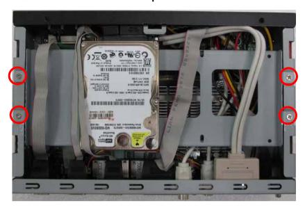
7. Push the Chassis shield towards the back then open it.
